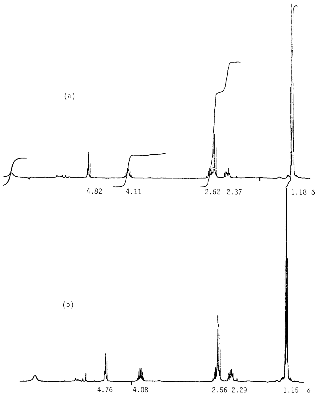
Fig. 2. NMR spectra of racemic 4-isopropylaminocarbonyl- \gamma -butyrolactone. (a) neat; (b) in presence of TFAE
